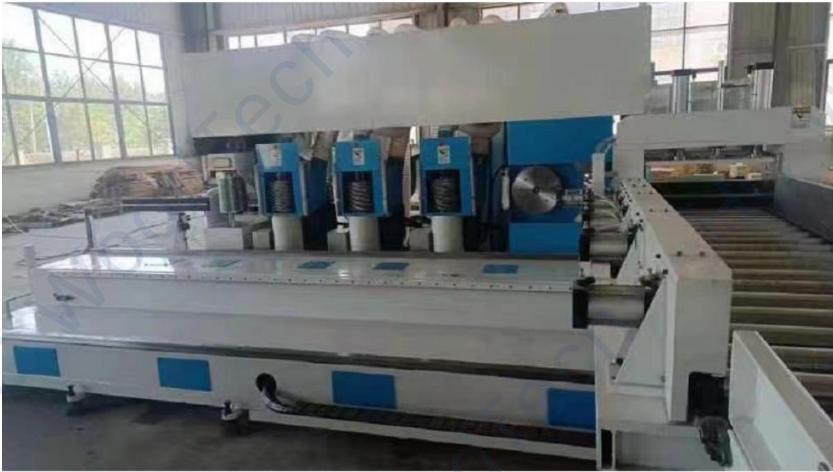
Finger-shaping machine and transfer area
