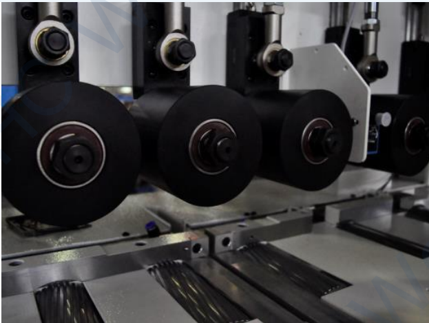
Saw blade area with scrap blow-off and pressure wheels
