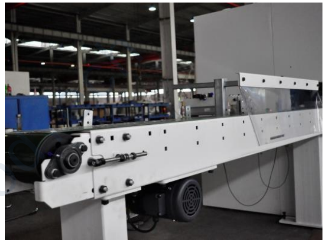
Extended infeed and defect marking table
